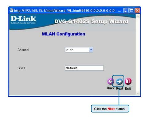
Enter the WLAN channel and SSID you want to use for your WLAN network. Initially, you can accept the default values and change the router's configuration later.
